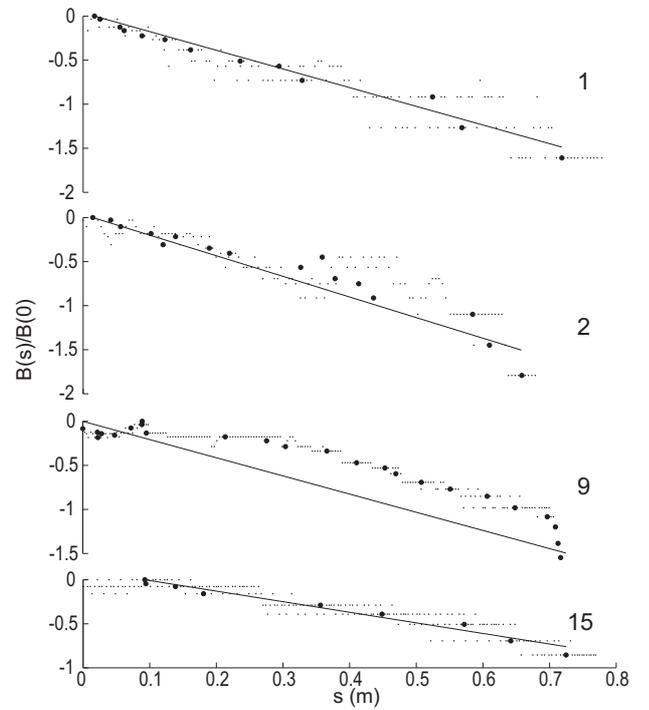
Figure 10: Logarithm of the ratio  $B(s)/B(0)$ , with versus the intrinsic coordinate,  $s$ , for the channels indicated in Figure 7.  $B(s)$  is channel width at  $s$ ,  $B(0)$  is width at channel inlet.
