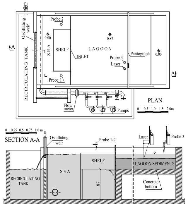
Figure 1: Sketch of the experimental apparatus
