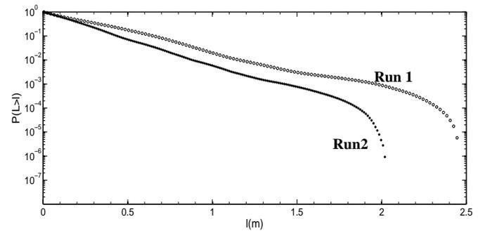
Figure 6: Probability distribution of unchanneled lengths for the channel network observed at the end of Run 1 and Run 2.
