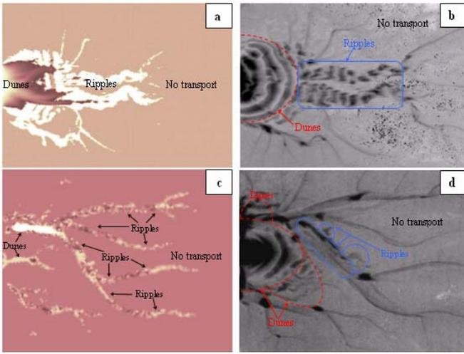
Figure 5: Spatial distribution of bed forms: (a, c) predicted through the criterion of Simons & Richardson (1966) applied to the computed values of  $R_p$  and  $\tau^*$  for Run 1 (a) and for Run 2 (c); (b, d) arising from experimental observations for Run 1 (b) and for Run 2 (d).
