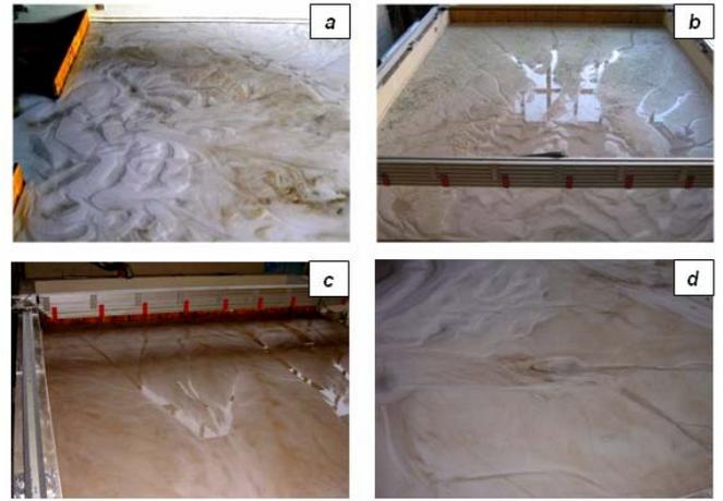
Figure 2: Lagoon topography observed in Run 1 after: a) 1200 cycles b) 6000 cycles and in Run 2 after: c) 6000 cycles; d) 7710 cycles.
