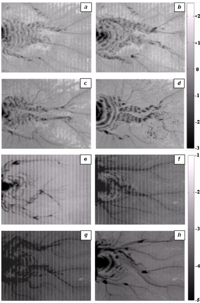
Figure 3: Distribution of bottom elevations measured within the lagoon in Run 1 after: a) 1650 cycles; b) 2900 cycles; c) 3910 cycles; d) 5950 cycles; in Run 2 after: e) 2200 cycles; f) 6270 cycles; g) 6845 cycles; h) 7700 cycles. Vertical bands are the consequences of changing tidal levels during the acquisition of the bathymetry. Elevations are referred to the initial uniform bottom elevation.
