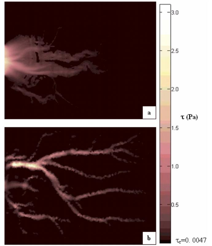
Figure 4: Spatial distribution of the excess Shields stress,  $\tau^* - \tau_{cr}^*$ , computed: (a) or the final configuration of Run 1 and (b) of Run 2. Both  $\tau^*$  and  $\tau_{cr}^*$  have been calculated using  $d_{50} = 0.8$  mm, as representative grain size of the adopted sediments.
