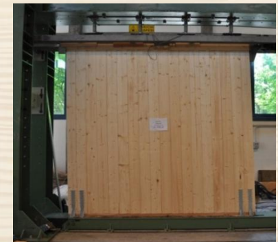
Cyclic tests of walls CNR IVALSA lab - 2014
